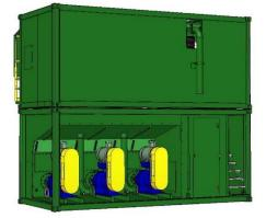
Each of the two modules of the SC150DP is built to the dimensions of a type 1CC 20-foot freight container, complete with ISO corner castings, which makes them easy to transport and handle on site. The shaker module has a heavy-duty hollow section frame, permanently enclosed on three sides and with a roof clad in marine quality plywood. A tarpaulin is fitted to the front in order to provide weather protection to the equipment and operator.
